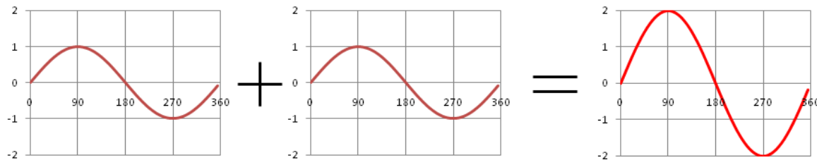
A. Two Equal Amplitude Waves Arriving In-Phase sum to Twice Amplitude
